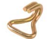
NH1000-7 2" Wire-Formed Closed Hook Breaking Strength: 5,000 lbs. Working Load Limit: 1,667 lbs.
