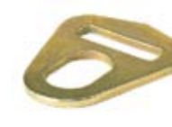
NH7936-1 2" Slotted Delta Ring, CHP rated Breaking Strength: 16,200 lbs. Working Load Limit: 5,400 lbs.
