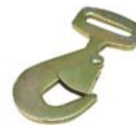
NH12009 2" Flat Snap Hook Breaking Strength: 10,000 lbs. Working Load Limit: 3,333 lbs.
