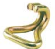
NH1000-6 2" Wire-Formed Closed Hook Breaking Strength: 10,000 lbs. Working Load Limit: 3,333 lbs.
