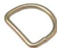
NH34025-14 1-3/4" D Ring Breaking Strength: 5,000 lbs. Working Load Limit: 1,667 lbs.
