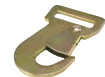
NH7900-1 2" Flat Snap Hook Breaking Strength: 6,000 lbs. Working Load Limit: 2,000 lbs.
