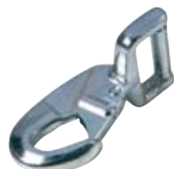
NH1211 2" Forged Snap Hook Breaking Strength: 10,000 lbs. Working Load Limit: 3,333 lbs.
