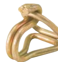
NH33210 2" Hook & Keeper Breaking Strength: 5,000 lbs. Working Load Limit: 1,667 lbs.
