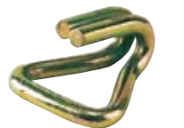
NH34031-10 1" Wire Closed Hook Breaking Strength: 3,000 lbs. Working Load Limit: 1,000 lbs.
