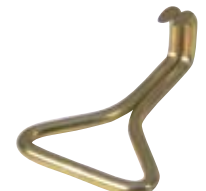
NH34031-7 1" Pallet Hook Breaking Strength: 2,000 lbs. Working Load Limit: 667 lbs.
