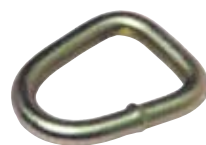
NH34025-50 1" Welded Delta Ring Breaking Strength: 5,000 lbs. Working Load Limit: 1,667 lbs.
